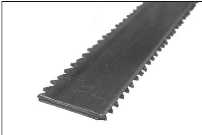
Figure 11. Blade ends stacked with teeth facing opposite directions.
